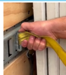
Insert top of clip first, rotate down to insert bottom, release lever to lock To remove clip, pull back lever, rotate clip in and pull out
