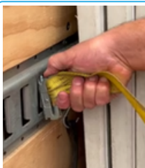
Insert top of clip first, rotate down to insert bottom, release lever to lock To remove clip, pull back lever, rotate clip in and pull out
