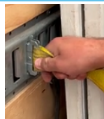
Insert top of clip first, rotate down to insert bottom, release lever to lock To remove clip, pull back lever, rotate clip in and pull out
