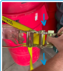
Pull ratchet assembly toward you to loosen
