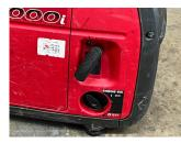
Hold the generator in place with one hand on the handle and pull the starter cord as quickly as you can
