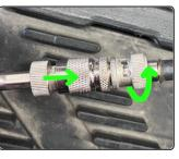
After making each connection, tuck the cables into the channels to protect the cables and connectors. Bump up one channel just before you move to the next mat.
